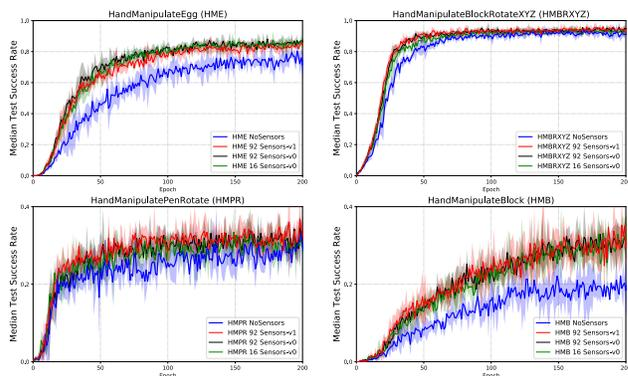
Fig. 3. Curves - median test success rate. Shaded areas - interquartile range [five random seeds]. Blue curves - learning without tactile information (NoSensors), red curves - learning with float-value tactile readings (Sensors-v1) from 92 sensors, black curves - learning with Boolean-value tactile readings (Sensors-v0) from 92 sensors, green curves - learning with Boolean-value tactile readings (Sensors-v0) from 16 sensor sub-groups.
