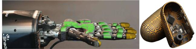
Fig. 1. Shadow Dexterous Hand equipped with fabrics-based tactile sensors in the palm and finger phalanges (indicated green) and fingertip sensors realized by Molded-Interconnect-Devices (indicated yellow) [4] [5]
