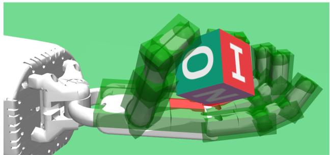
Fig. 2. 92 touch sensors covering the Shadow Dexterous Hand model. This is a technical visualization to represent the essence of our model. Red sites represent activated touch sensors, where a block is pressing against the touch sensitive area. Green sites represent inactive touch sensors. A video demonstration of the extended environments can be found at <https://rebrand.ly/TouchSensors>
