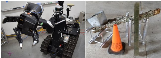
Figure 1. Left: Army Research Lab’s ‘RoMan’ mobile manipulation platform with broken proximal joint on Robotiq 3-finger Gripper. Right: Example debris pile of massive objects, where lifting two or more items exceeds manipulator payload limits.
